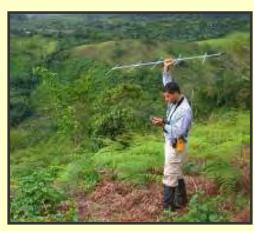
Multi-element Yagi antennas are one of the most commonly used antennas in radio-tracking
